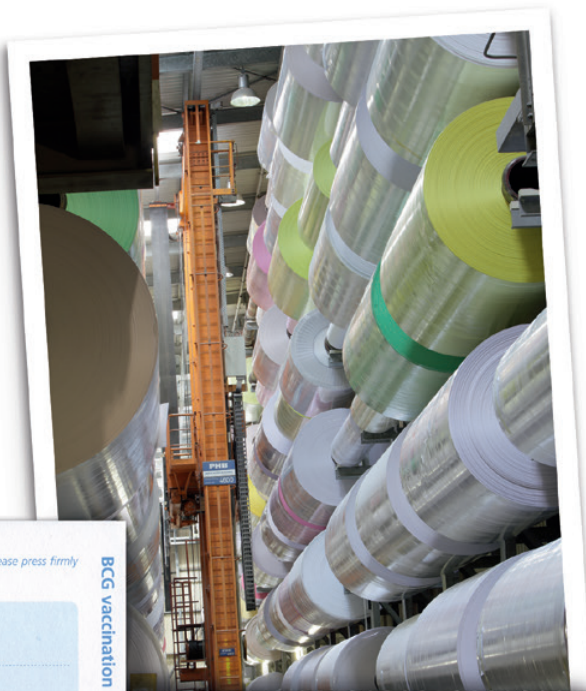
High racking for interim storage of the jumbo rolls. Fully automated and air conditioned.
